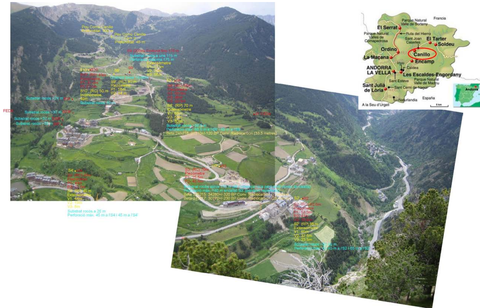
Figure 1: Inventory of field data and monitoring on the El Forn giant landslide (in Catalan), in red piezometers, in yellow extensometers, in blue soundings and bedrock contact, some other data in red and yellow related to groundwater wells and hydroelectric pipeline, thanks to Xavier Planas i Batlle from the Andorra Government.
